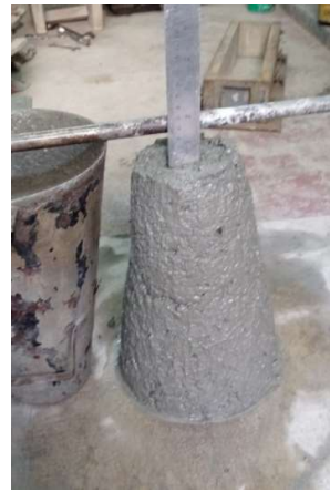
Polypropheline @45min slump-45mm
