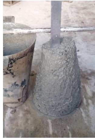
Optica fibers @45min slump – 50mm
