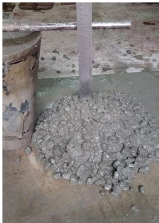
Control mix Initial slump – 195mm
