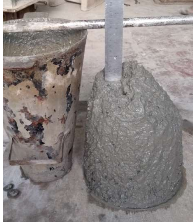
Optica fibers Initial slump – 100mm
