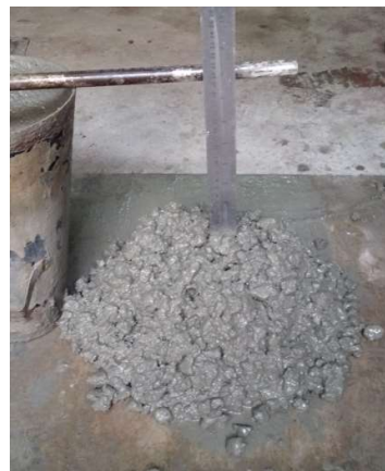
Control mix @45min slump -190mm
